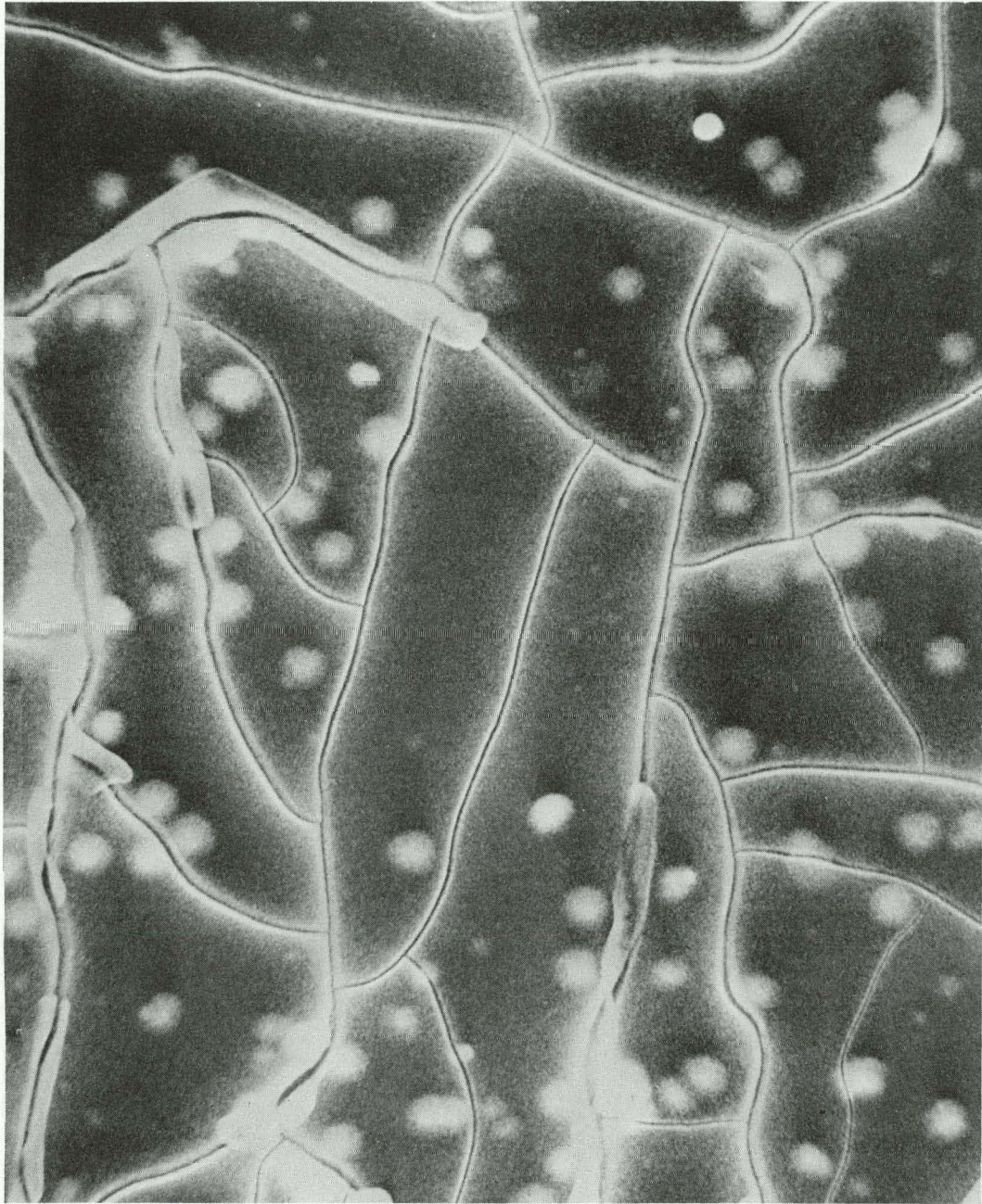
Figure 4.23. SEM photograph of the cracked surface on a strongly reduced \text{Na}_{0.6}\text{WO}_3 crystal which had been previously anodized. Aside from the cracks, the surface is very smooth except for the small round particles which are of unknown composition. The magnification is 6,000X
