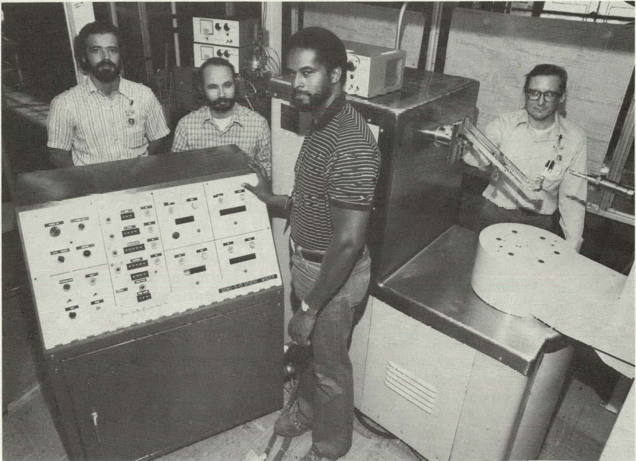
FIG. 18. The new sphere winder with sphere arm and spindle at right, resin mix and filament delivery system in background, and control system at left. Participants in development of the machine are (left to right) Dennis Silva and Ken Waltjen, both of the Electronics Engineering Department, and Leon Newton and Bob Sherry, both of the Mechanical Engineering Department.
