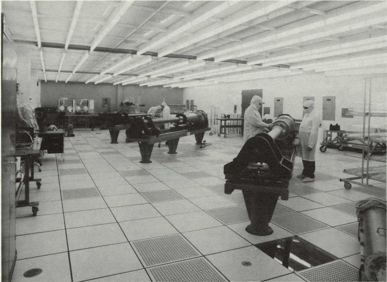
FIG. 12. Class 100 clean room used for cleaning, assembling, and inspecting rod and disk amplifiers.
