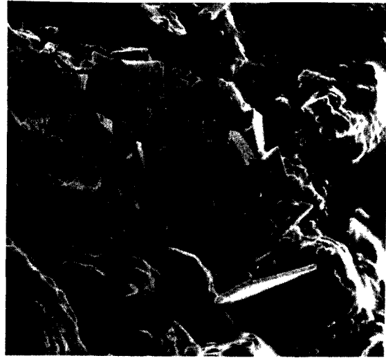
Fig. 13: SEM-photograph of newly built idiomorphic magnetites at UCG-like conditions: flowrate 2 kg/h, air/steam-mixture 1:1, T=600^{\circ}\text{C} , \bar{p}=40 bars.
