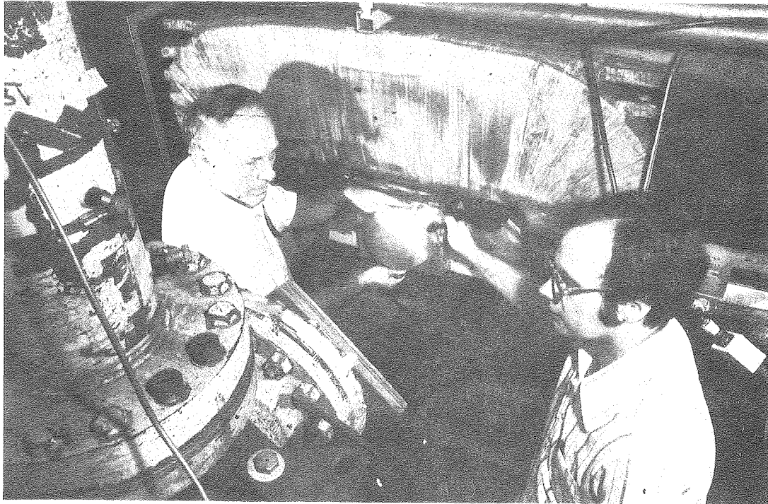
LBL physicists William Wenzel and David Fancher at work on prototype time projection chamber.
