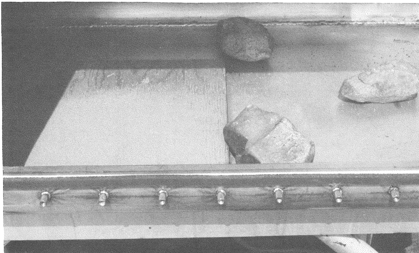
FIGURE 3. Spilled Powder Pattern After Impact by Three Rocks
