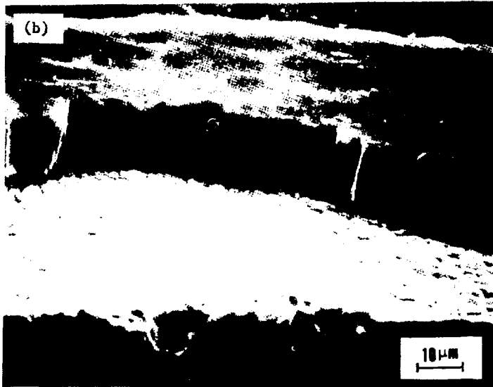
Figure 1-14. Scanning electron micrographs (SEMs) of fractured edges of (a) a sooty deposit on a graphite substrate, and (b) a dense adherent coating on a stainless steel substrate.
