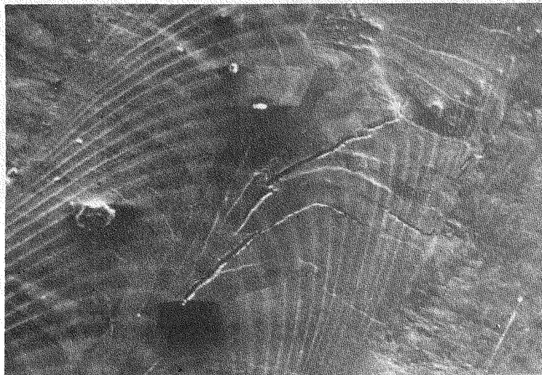
C. SEM PHOTO OF CRACKS ON INSIDE WELD SURFACE, X80
