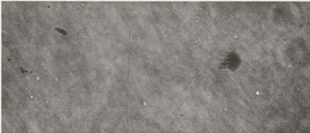
Figure 14 Laser Shadowgraph #3, 520-Micron Gold Microsphere and Isodensitometer Trace (8B159)
