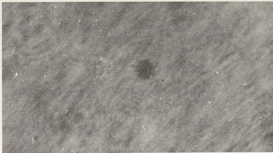
Figure 13 Laser Shadowgraph #3, 650-Micron Gold Microsphere and Isodensitometer Trace (8B158)
