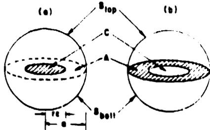
Fig. 1 Cracked spheres. The interior crack (a) has free boundaries; the peripheral crack (b) is fluid-filled. The equatorial plane is divided into a circle (C) and an annulus (A). The top and bottom hemispheres are called  $S_{top}$  and  $S_{bot}$ .
