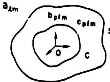
Fig. 2 A void (surface C) within an inclusion (surface S) immersed in a fluid. The displacement outside S consists of a plane wave plus outgoing partial waves (coefficients  $a_{lm}$ ); inside S it is expanded in regular (coefficients  $b_{plm}$ ) and irregular (coefficients  $c_{plm}$ ) eigenfunctions of the elastic wave equation. The origin of coordinates is always taken inside C.
