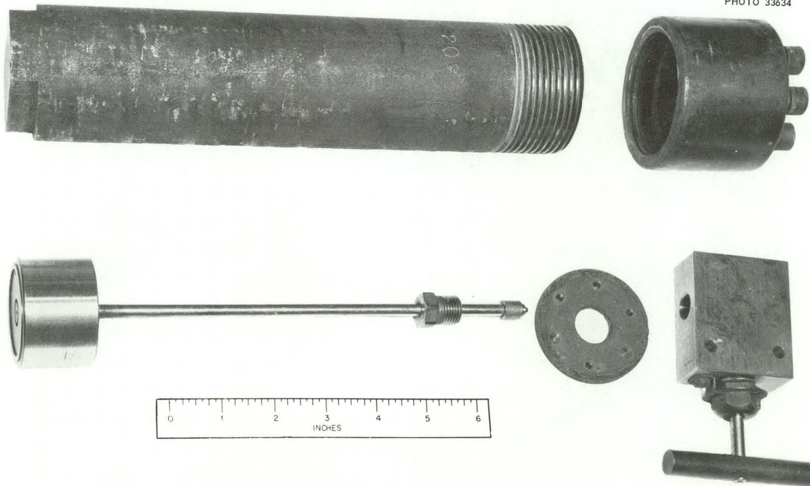
Fig. 5. Autoclave and Accessories Used in APPR Corrosion Testing Program.
