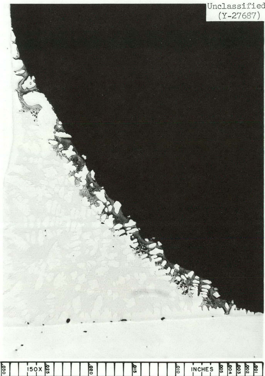
Fig. 10. Corrosion of Brazed Fillet of Coast Metals N.P. Joined to Type 304L Stainless Steel After 12 Months in Static 565°F, 1200 psi Distilled Water Containing 50 cc H 2 /liter and 1 cc O 2 /liter. Etchant: 10% oxalic acid.
