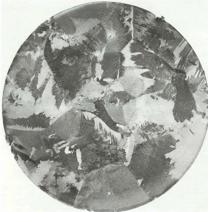
Fig. 2. Same Zirconium Specimen Shown in Fig. 1 After Polishing and Etching. 7X.
