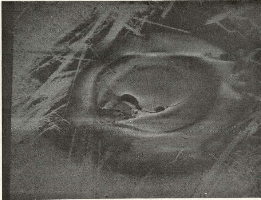
FIGURE 7. Damage Site Containing Only Iron. Sample VK-6. Magnification 85X.
