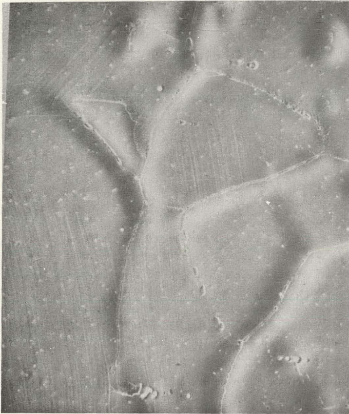
FIGURE 15. Surface Striations on Flashed Sample. Sample VH-10. Magnification 500X.
