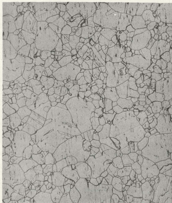
FIGURE 2. Microstructure of Sample Solution Treated at 1050 °C, then Stabilized at 850 °C. Magnification 100X.
