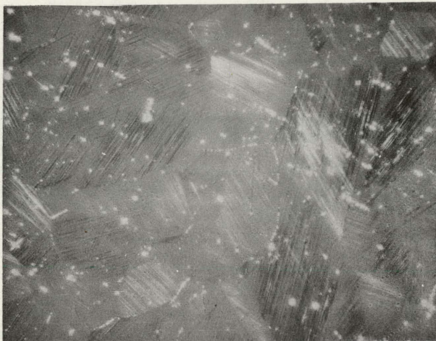
FIGURE 17. Different Orientations of Striations Within Each Grain. Sample VK-1. Polarized Light. Magnification 400X.
