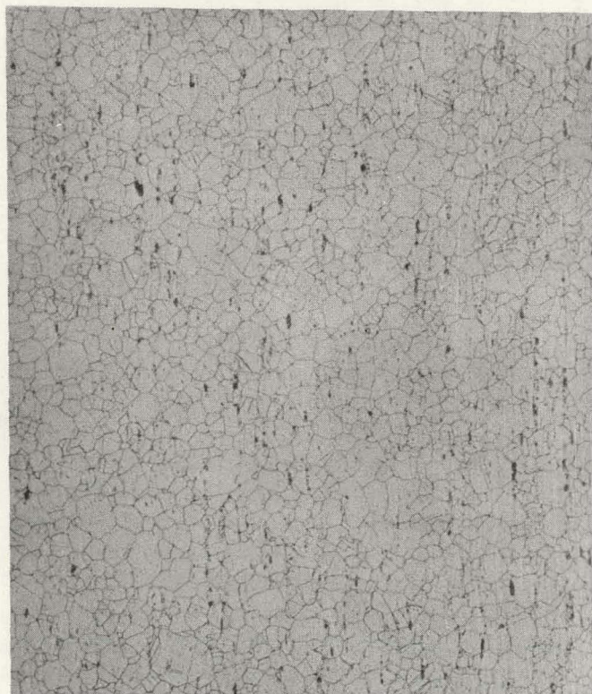
FIGURE 1. Microstructure of As-Received Type 304 Stainless Steel. Magnification 100X.
