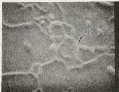
FIGURE 14. Comparison of Matrix and Grain Boundary Inclusions in a Stabilized, Electropolished and Chemical Polished Sample (a) Before, and (b) After Flashing. Sample VH-5. Magnification 300X.
