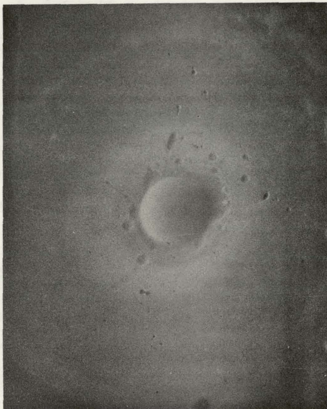
FIGURE 12. Damage Site Containing Iron, Copper, and Zinc. Sample VH-6. Magnification 190X.
