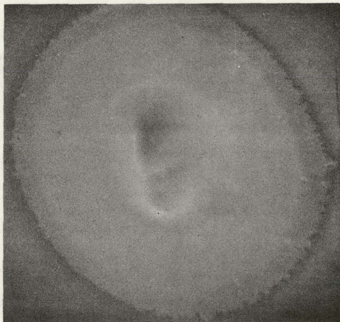
FIGURE 6. Damage Site Containing Only Iron. Sample VH-3. Magnification 525X.
