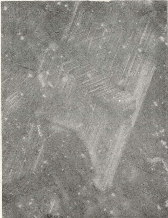
FIGURE 19. Change in Crystallographic Orientation of Striations at a Twin Boundary. Sample VH-2. Polarized Light. Magnification 400X.
