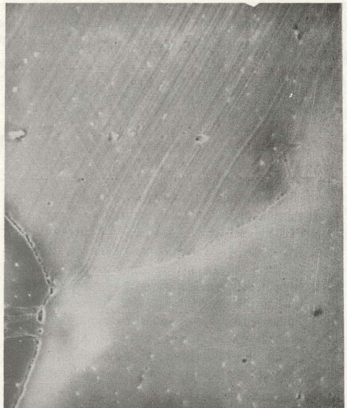
FIGURE 16. Surface Striations and Grain Boundary Precipitates. Sample VH-10. Magnification 2000X.
