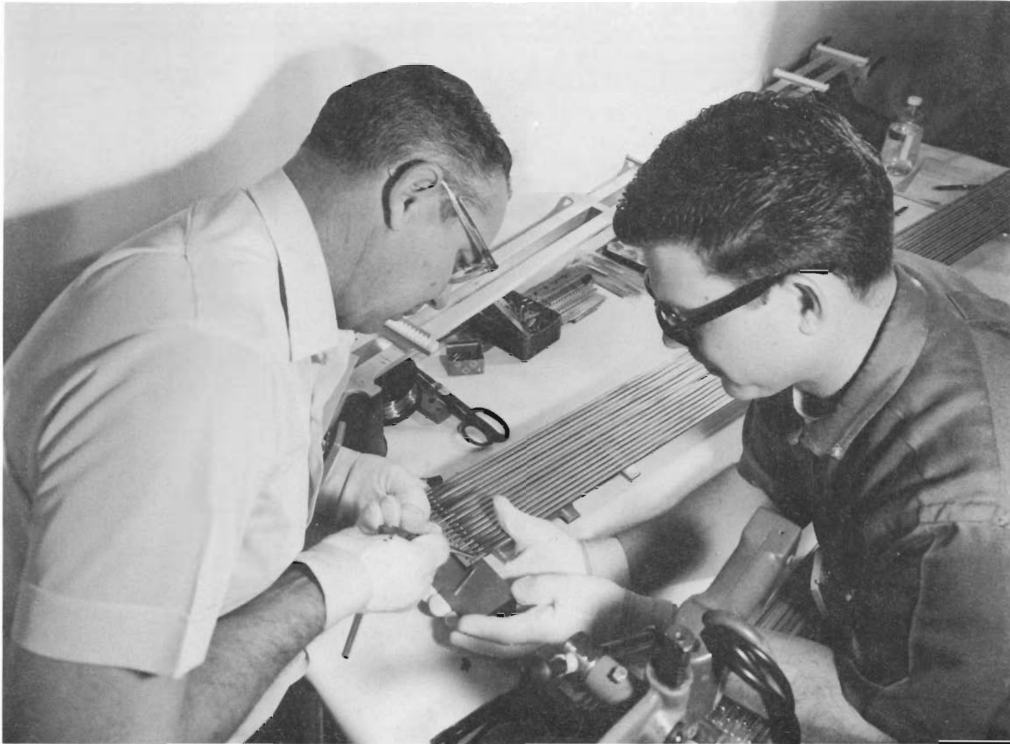
FIGURE 44. Fastening Rows of Fuel Pins to Grid Strips
