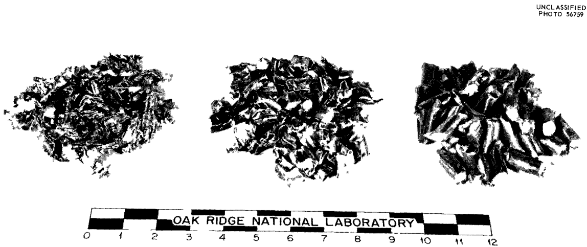
Fig. 1. 19. Comparison of Product from Shearing ORNL Mark I Fuel into 0.25-, 0.50-, and 1-in. Lengths.
