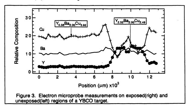
SEM showed adifference in target surface morphology for the laser irradiated (melted) region that in many cases exhibits a columnar regrowth structure. These results suggest that during the ablation process, the incongruently melted zone is larger than the congruently evaporated layer (etch depth). Additionally, microprobe analysis of the target surface unexposed by the laser also showed a relative Y deficiency. This is due to redeposition of Cu and Ba rich particulates from the ablation plume.
