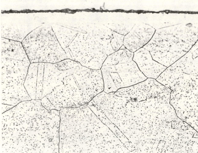
Figure 2.10 Optical Photomicrographs Showing Surface Condition and Etched Subsurface Microstructure of HD-556 after Approximately 1000 Hour Exposure in Controlled Purity He at (a) 750°C and (b) 850°C.
