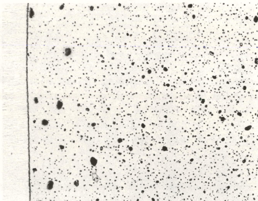
Figure 2.30 Optical Photomicrographs of Yd-Ni Exposed in Controlled Purity He for (a) 1000 Hours at 750°C and (b) 1104 Hours at 850°C.
