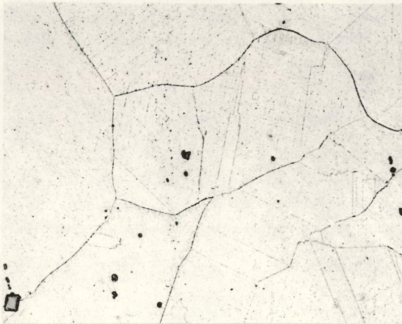
Figure 2.1 Optical Photomicrographs Showing Etched Internal Microstructure of Alloy 800H after Exposure in Controlled Purity He for (a) 1000 Hours at 750°C and (b) 1104 Hours at 850°C.
