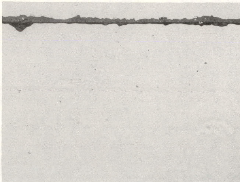
Figure 2.19 Optical Photomicrographs Showing Surface Condition (a) and (b), and Etched Subsurface Microstructure, (a) Only, of HK-40 after ~1000 Hour Exposure in Controlled Purity He at (a) 750°C and (b) 850°C.
