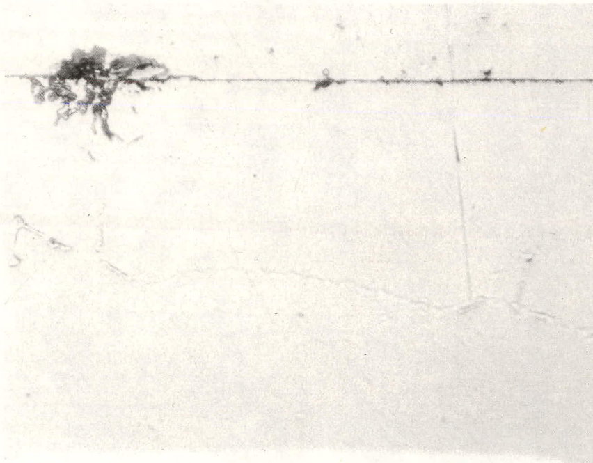
Figure 2.40 Optical Photomicrographs of IN-738 Exposed in Controlled Purity He for (a) 1000 Hours at 750°C and (b) 1104 Hours at 850°C.
