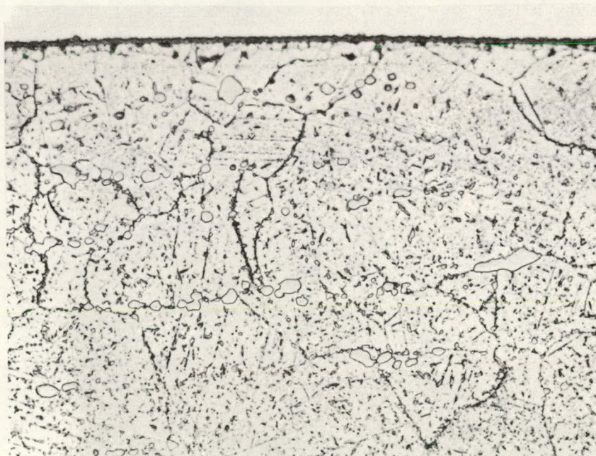
Figure 2.17 Optical Photomicrographs Showing Surface Condition and Etched Subsurface Microstructure of Hastelloy X after Approximately 1000 Hour Exposure in Controlled Purity He at (a) 750°C and (b) 850°C.
