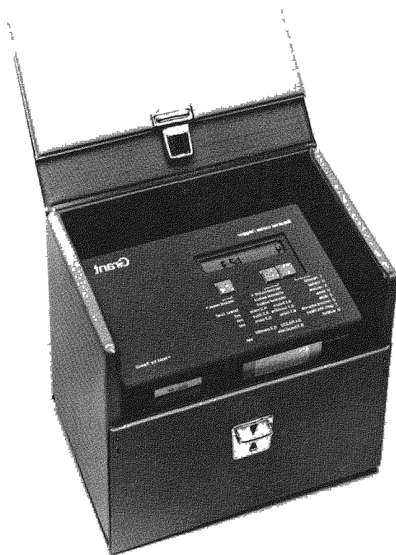
Figure 7. Digital Magnetic-Field Logger Uses the Same Pick-up Coil System as Described in Figure 6, with a Preamplifier Incorporating an Rms Module, Which Allows the Vector Sum to be Recorded in Parallel with the Three Spatial Components.
