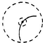
Figure 6.2: Schematic drawings of typical heavy lepton events for various ranges of \Delta m . Straight lines are heavy leptons, curved lines are their low-energy daughters, and diamonds mark decays. The dashed circles represent the inner and outer radii of the TPC.
