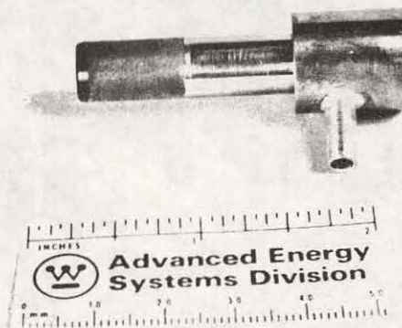
C) Cooling Channel Extension
