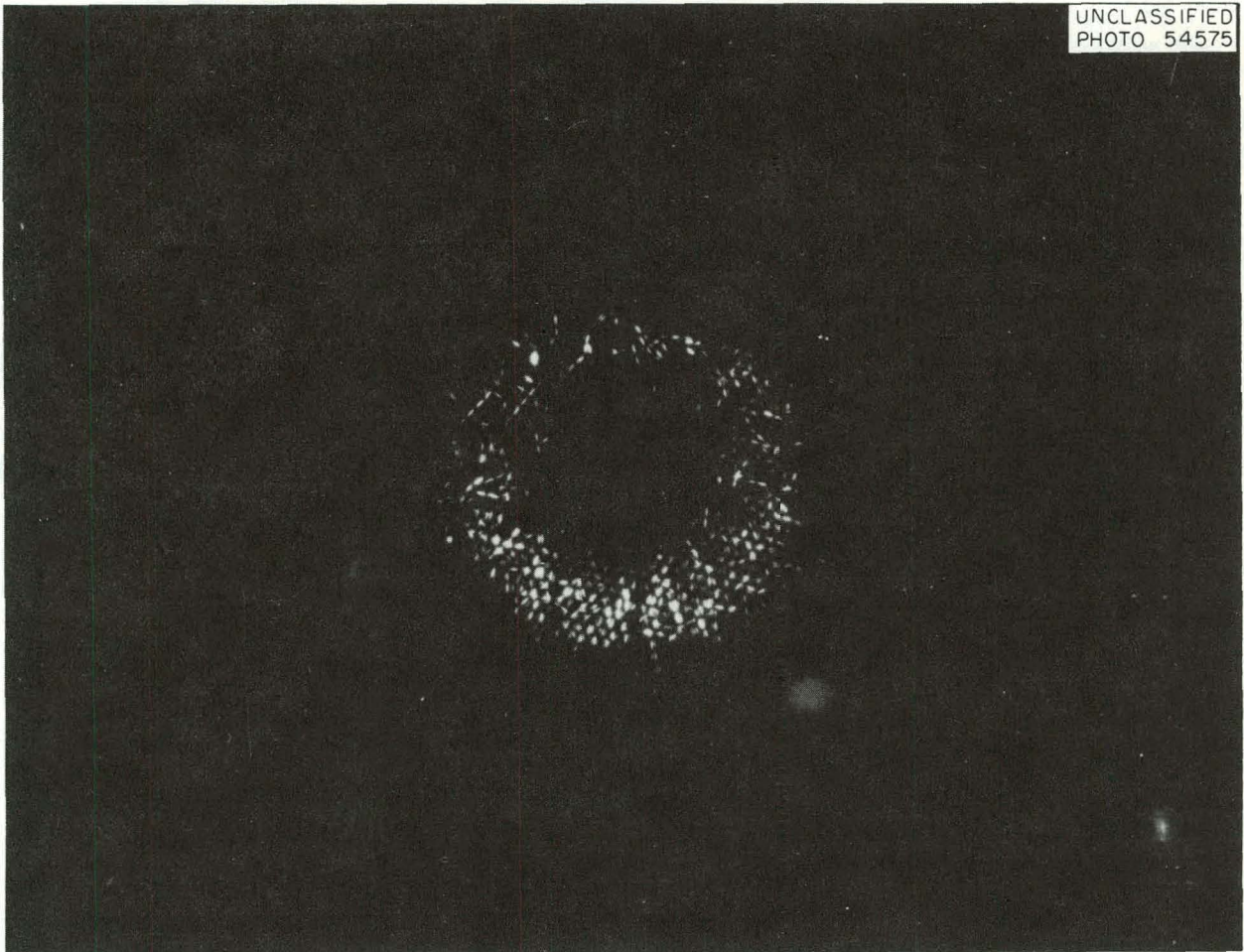
Fig. 3.1. Incandescent Molybdenum Powder Outlining the Hot Electron Plasma in the Resonant Magnetic Field Region.
