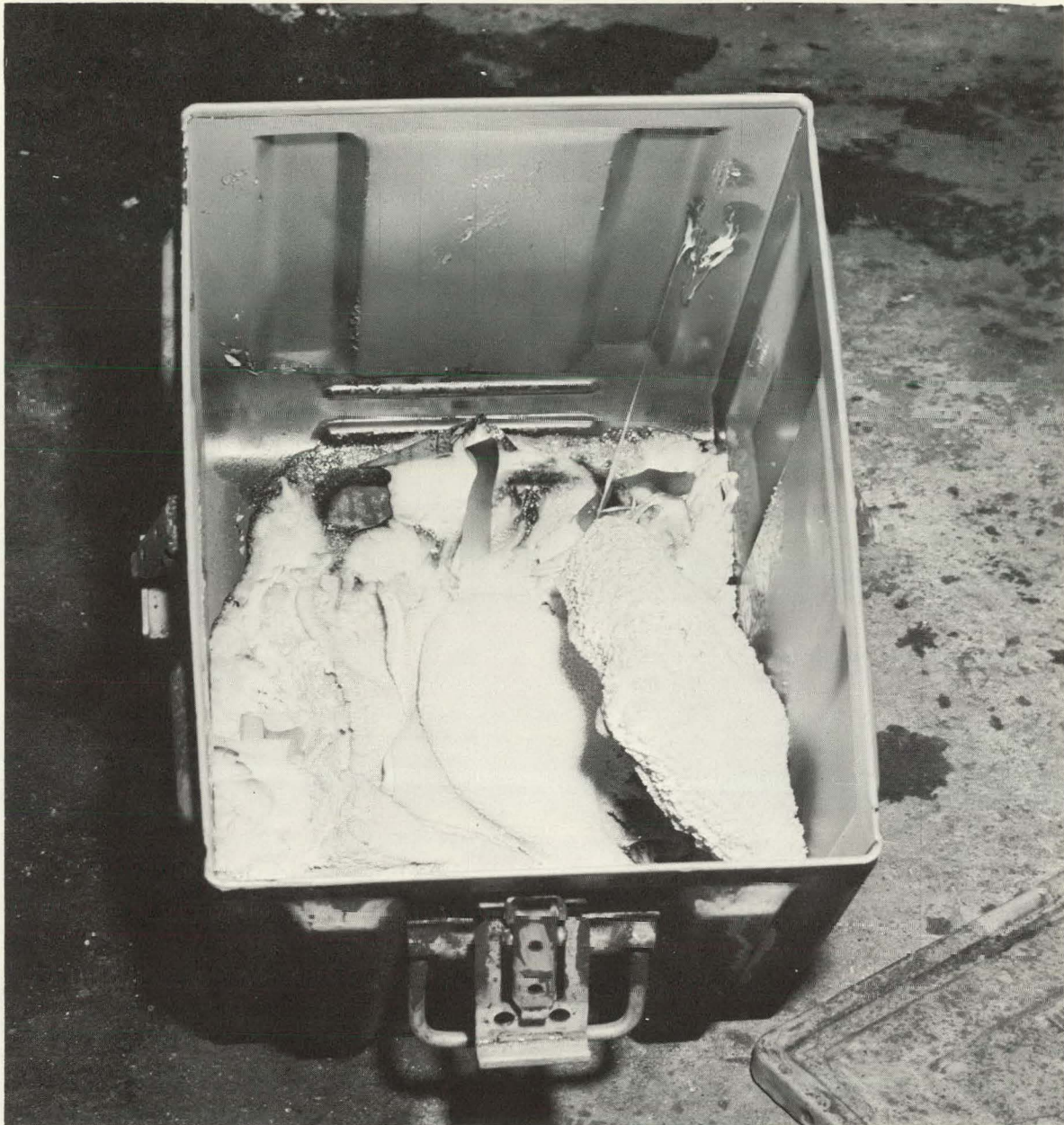
Figure 7. POLYSTYRENE FOAM CONTAINER MELTED DURING FIRE.
