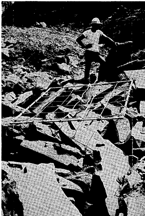
Fig. 29. Blasted rock from PB-5 (1-ft 2 grids).
