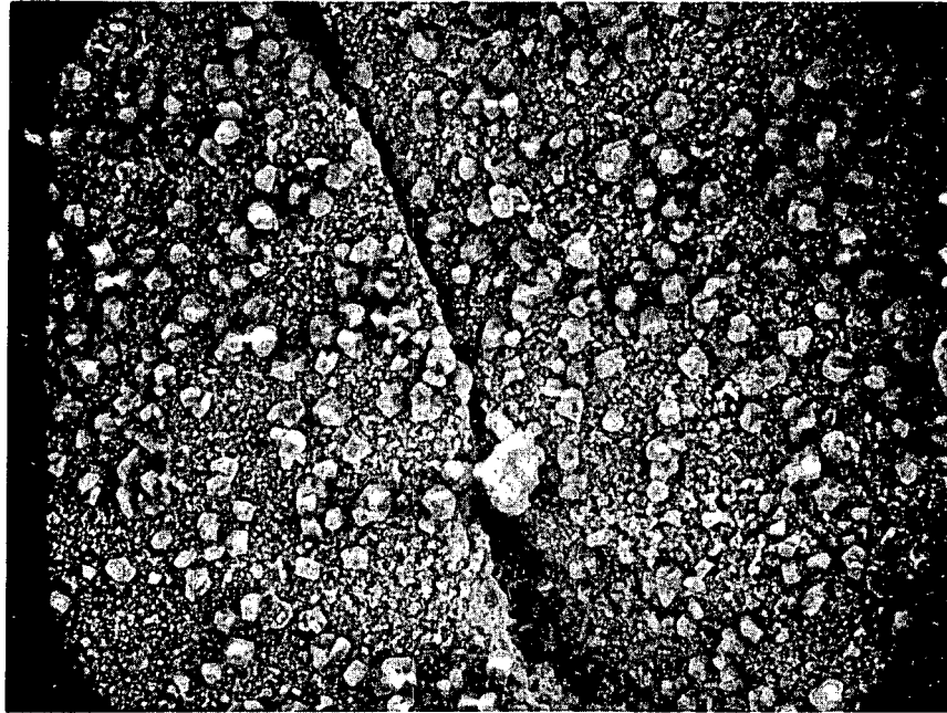
Figure 3-66. Second-stage nozzle fifth cooling passage inside surface showing fissure in the oxide layer inside the passage (magnification 500X)
