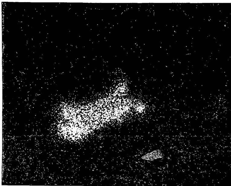
Figure 3-71. X-ray backscatter of sodium in area 1 of the second-stage nozzle (magnification 4000X)
