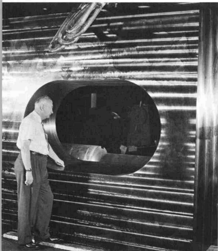
Figure 8. Window for 80-in. liquid hydrogen bubble chamber magnet. This window serves as part of the magnetic circuit and also forms part of the vacuum chamber. The opening allows the hydrogen chamber to be illuminated and photographed.
