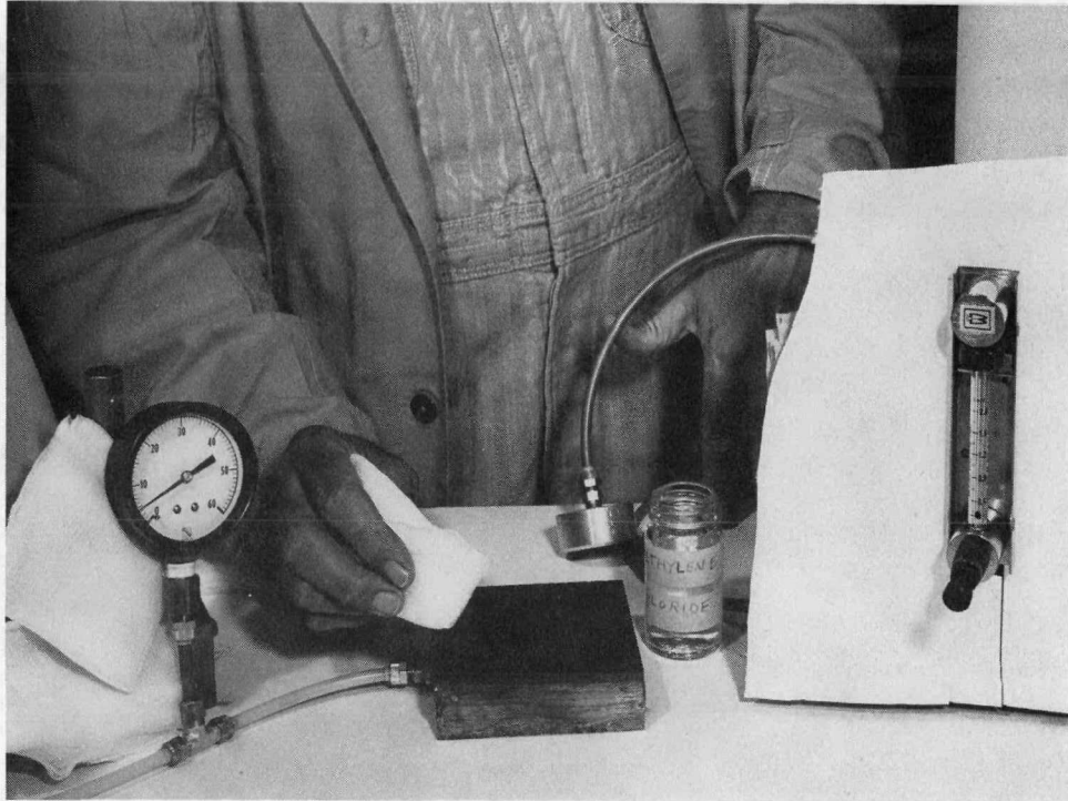
Figure 24. IMPREGNATION PROCEDURE. (Rewiping the Bearing Surface)
