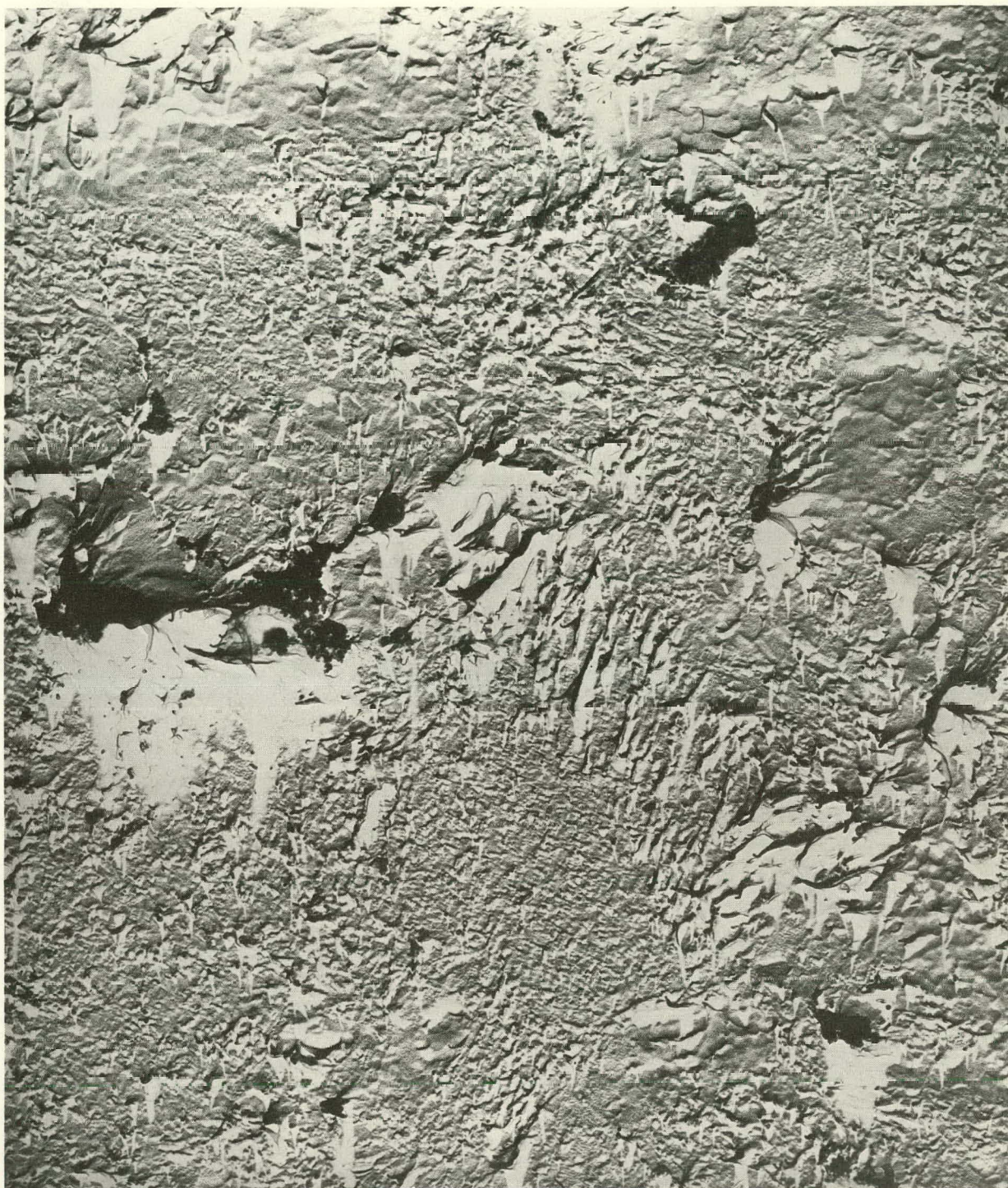
Fig. 3--Electron micrograph of an annealed fuel-matrix graphite. No cathodic etching. Carbon replica, negatively shadowed with Pd. Longitudinal section.
