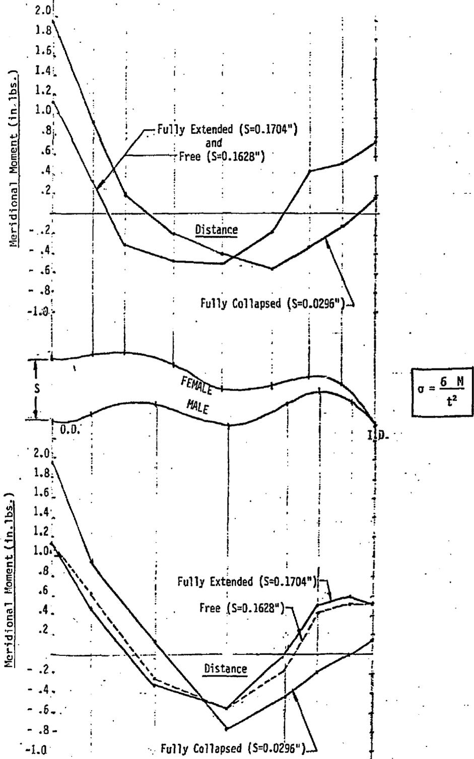
Figure 5. Meridional Moment Versus Radial Distance (Large Bellows - 0.009" Thickness)
