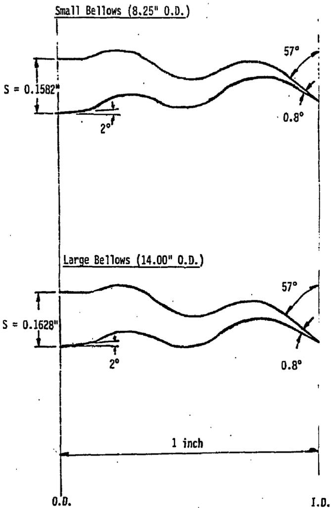
Figure 2. Bellows Geometry Modelled
