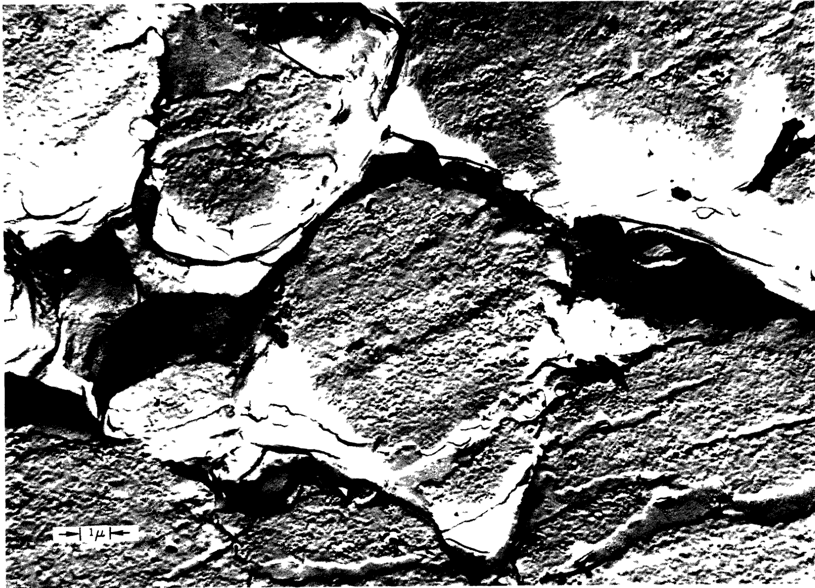
Figure 6. Intergranular Failure in 405 Stainless Steel With 4 \times 10^{-5} Atom Fraction Helium, Tested at 750°C (Electron Fractograph)
