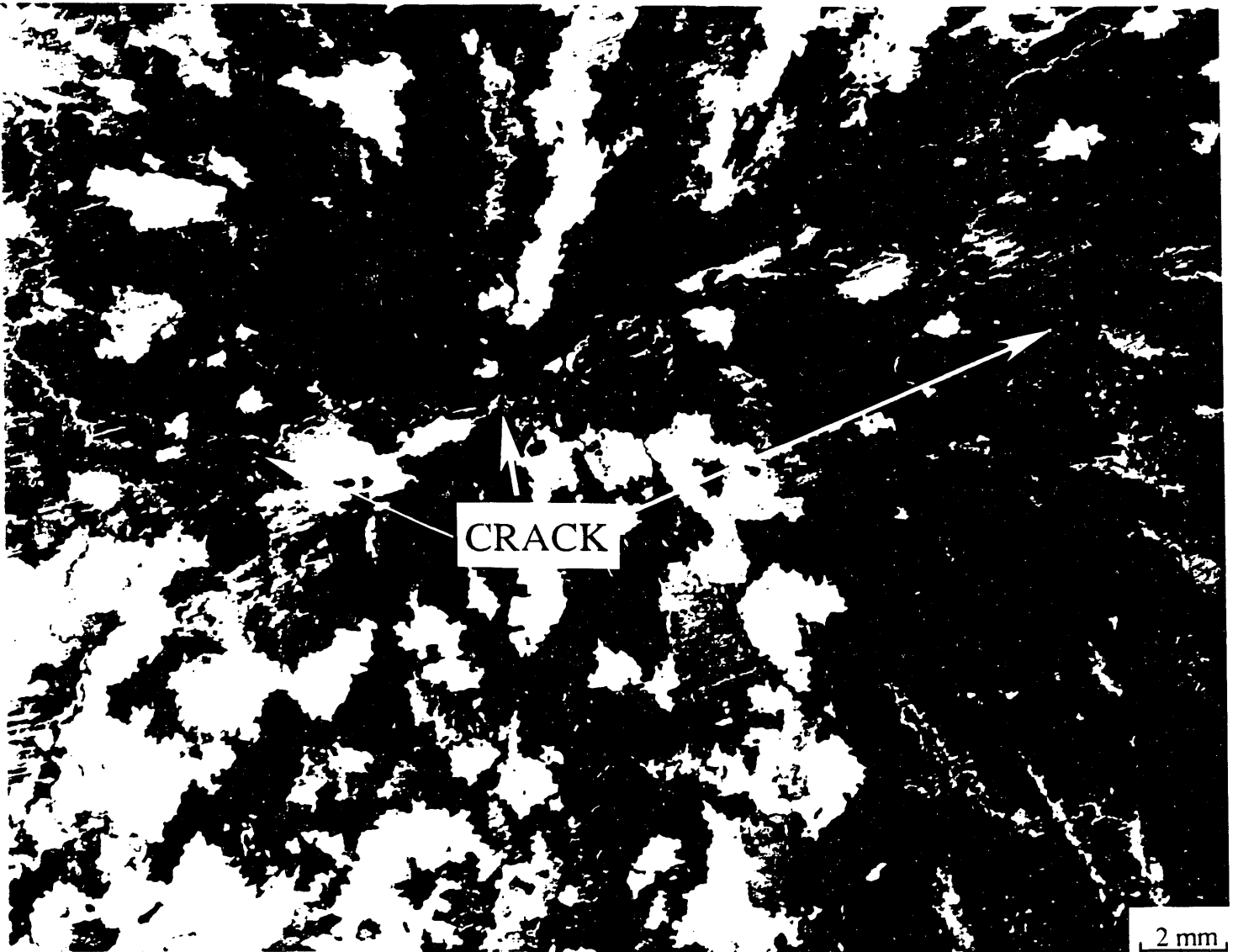
Fig. 5. Higher-magnification photograph of a macroetched section of a 403-mm-diam, electroslag-remelted ingot of IC-218LZr. Note the cracks.
