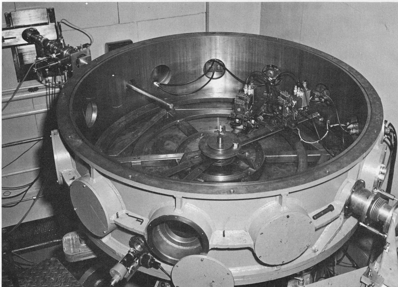
Fig. II.D-5. Photograph of the 60-in. scattering chamber at the present cyclotron. Four remotely-controlled detector arms are shown, with detector systems mounted on two of them. The target wheel is normally mounted on the central spindle.
