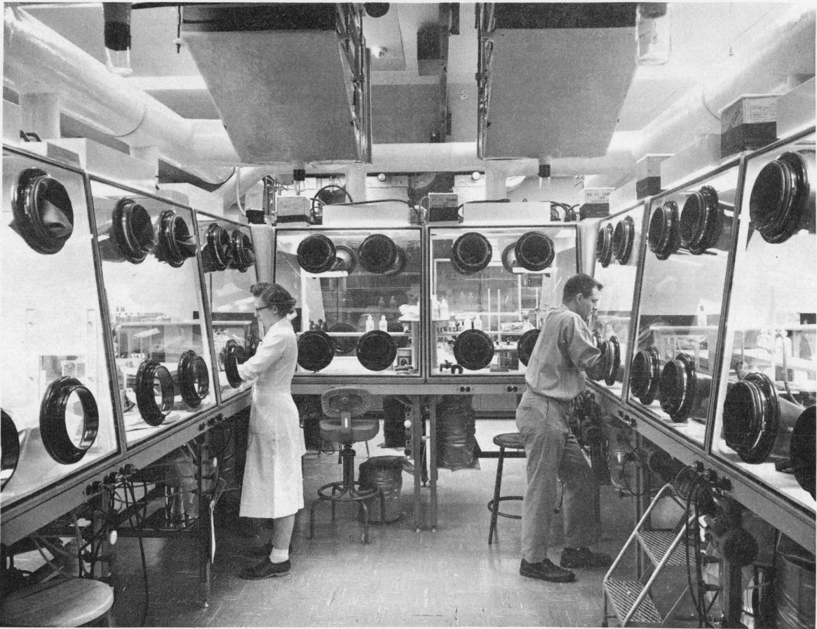
Fig. II. E-2. Typical alpha-activity laboratory with glove-box lines.
