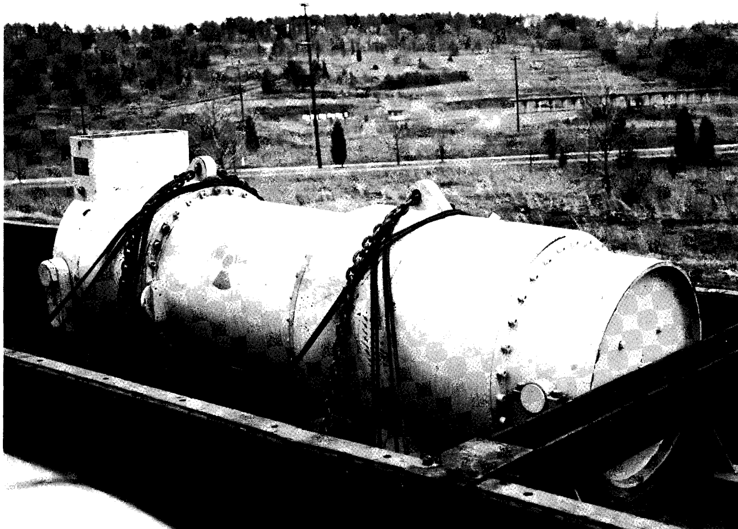
Fig. 5.2. SRE core I fuel shipment in 30 ton carrier (38" dia x 12'-7" long). Received at Y-12 spur track of Oak Ridge National Laboratory from Atomics International, Conoga Park, California.
