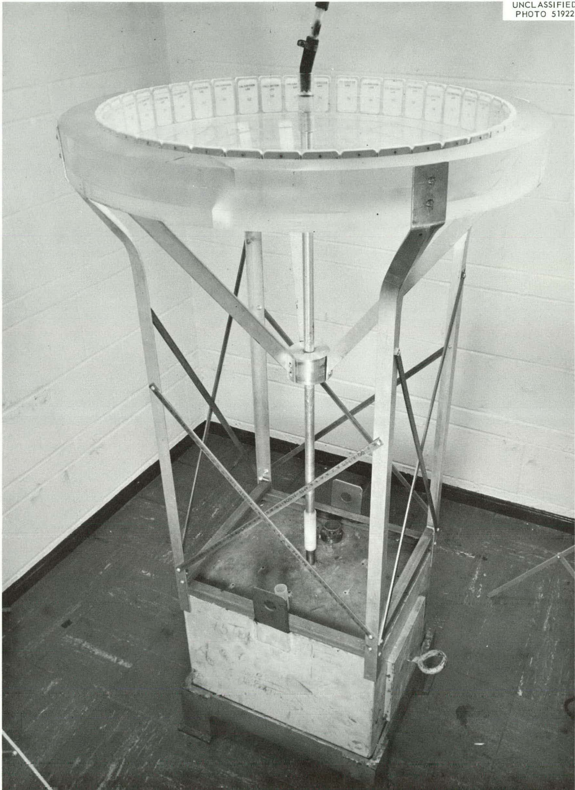
Fig. 12. Radium-gamma calibration ring.
