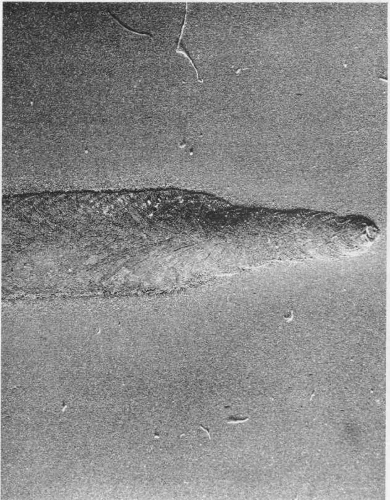
Fig. 4.8 - Pitting at Edge of Weld after Huey Test (15X)
