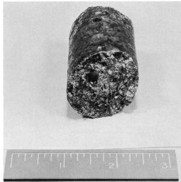
Figure 86. LiH-ZrH Aggregate Cast in a Titanium Tube
