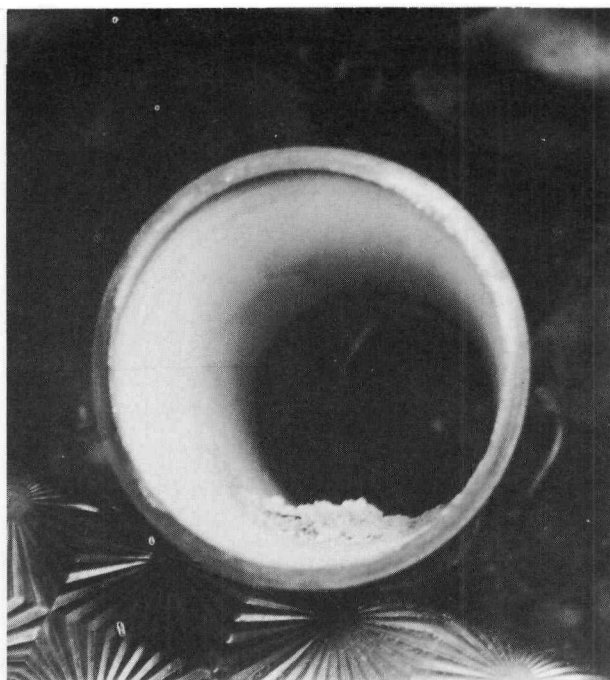
Figure 88. Granular Deposits in NaK Pipe
