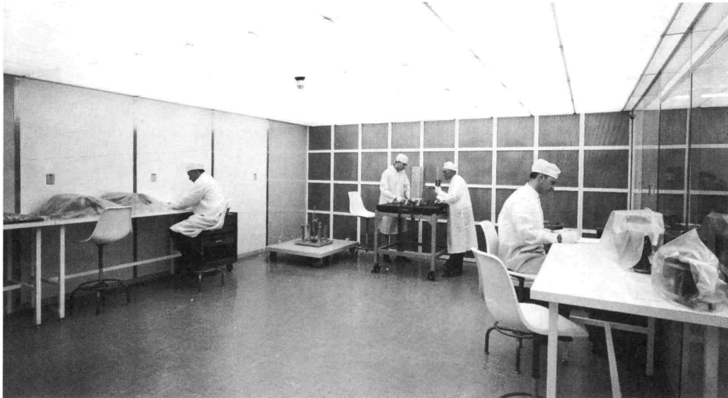
Figure 105. Prefabricated Laminar-Flow Clean Room, Interior View
