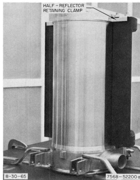
Figure 117. S8DS Tooling Vessel, Z-Half Reflector Clamped to Reactor Core Vessel
