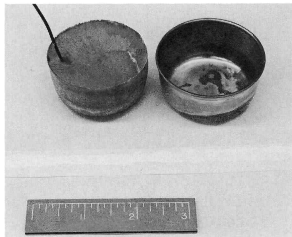
Figure 87. Released Casting and Titanium-Coated, Stainless-Steel Mold
