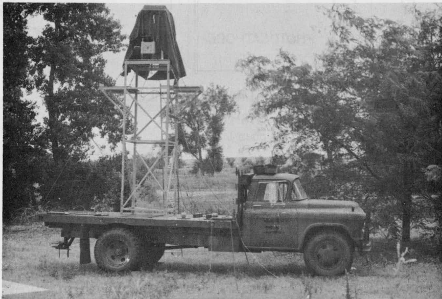
Fig. II B7 Mobile detector cart for long flight path work. A housing of boxed paraffin on top of the tower provides local shielding around the detector. The top of the tower is equipped with a turntable to facilitate alignment of the detector.
