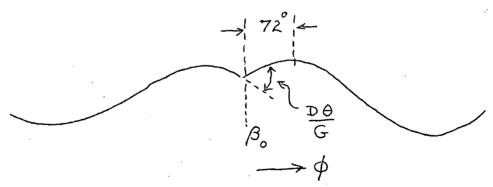
for v = 6.4 with the usual betatron form  $\frac{\beta_1^{\frac{1}{2}}}{\beta^2} \cos{(\phi - \phi_0)}$ . For a closed magnet, a positive D gives outward bend as in diagram
