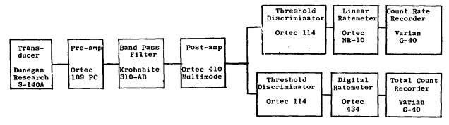
Fig. 4 - Acoustic Emission Equipment, Group Number One.
