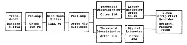
Fig. 5 - Acoustic Emission Equipment, Group Number Two.
