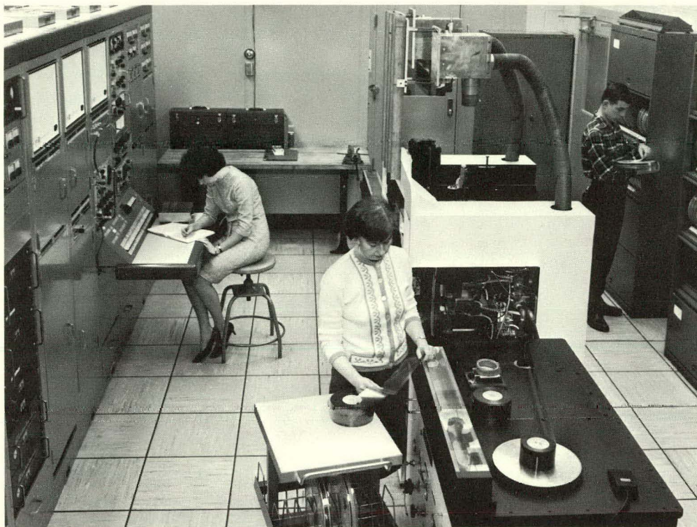
Figure 8. The BNL 70-mm Flying-Spot Digitizer, which has recently completed its first high-volume experiment and has contributed to the knowledge of the dipion mass spectrum near 1700 MeV.
