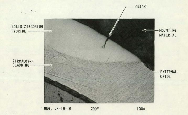
Figure 2–6. Part of Solid Hydride Area Containing External Crack, 18 Inches from the Bottom of Rod JX
