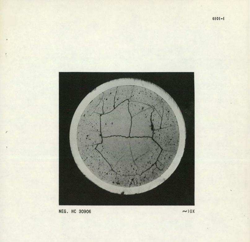
Figure 2–8. Macrograph of Transverse Section of Rod IM, 12.25 Inches from the Bottom the pellet surface was unusually large compared to that observed in the nonfailed rods of similar power history.
