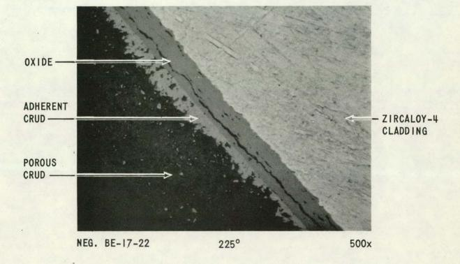
Figure 2-3. Adherent and Porous Crud and Oxide on Outer Surface of Rod BE, 17 Inches from the Bottom
