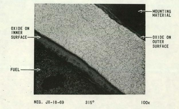
Figure 2-7. Oxide on Both Outer and Inner Surfaces of Rod JX, 18 Inches from the Bottom
