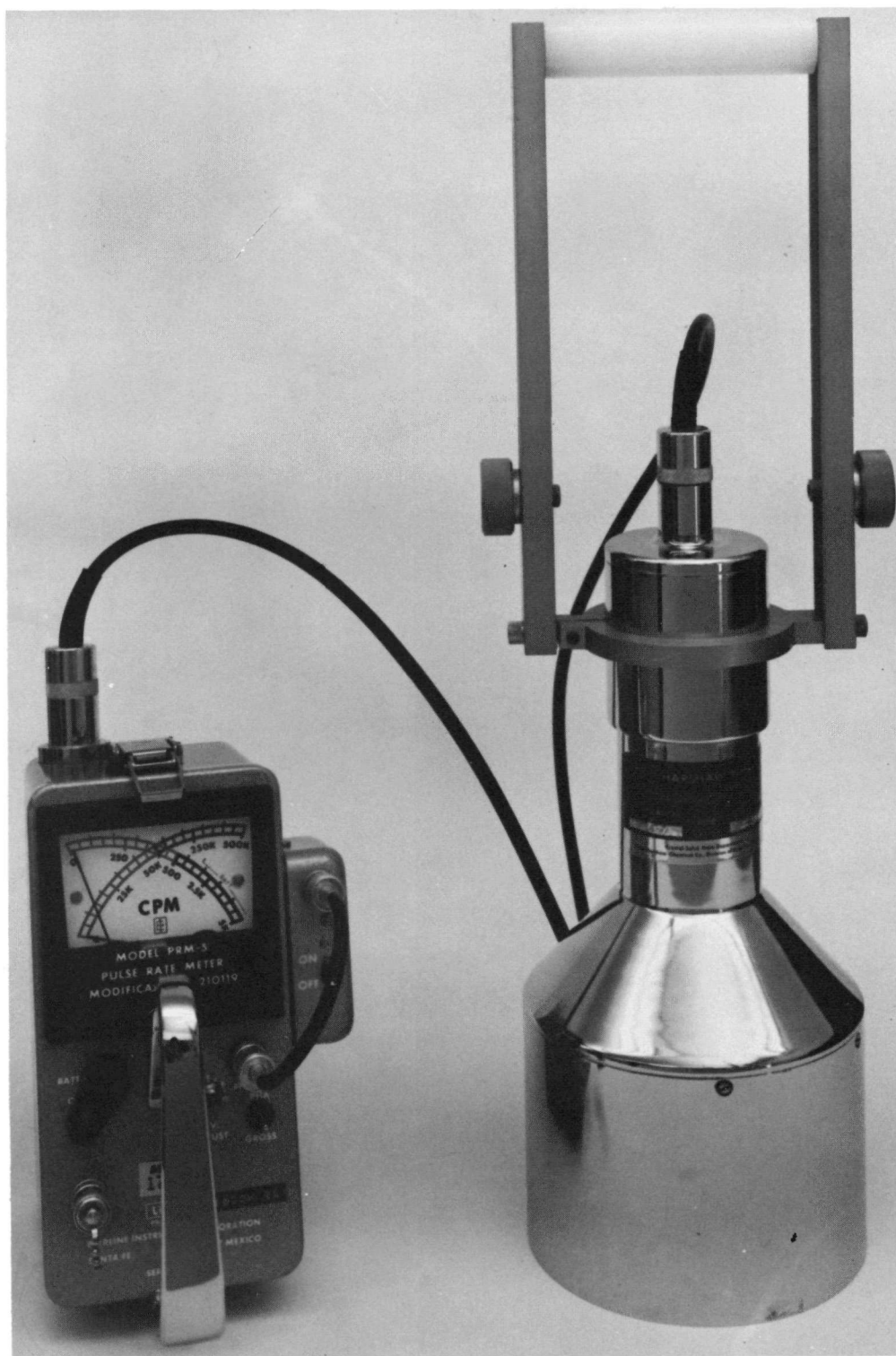
Fig. 1. FIDLER detector and pulse-rate meter used for plutonium surface-contamination surveys.
