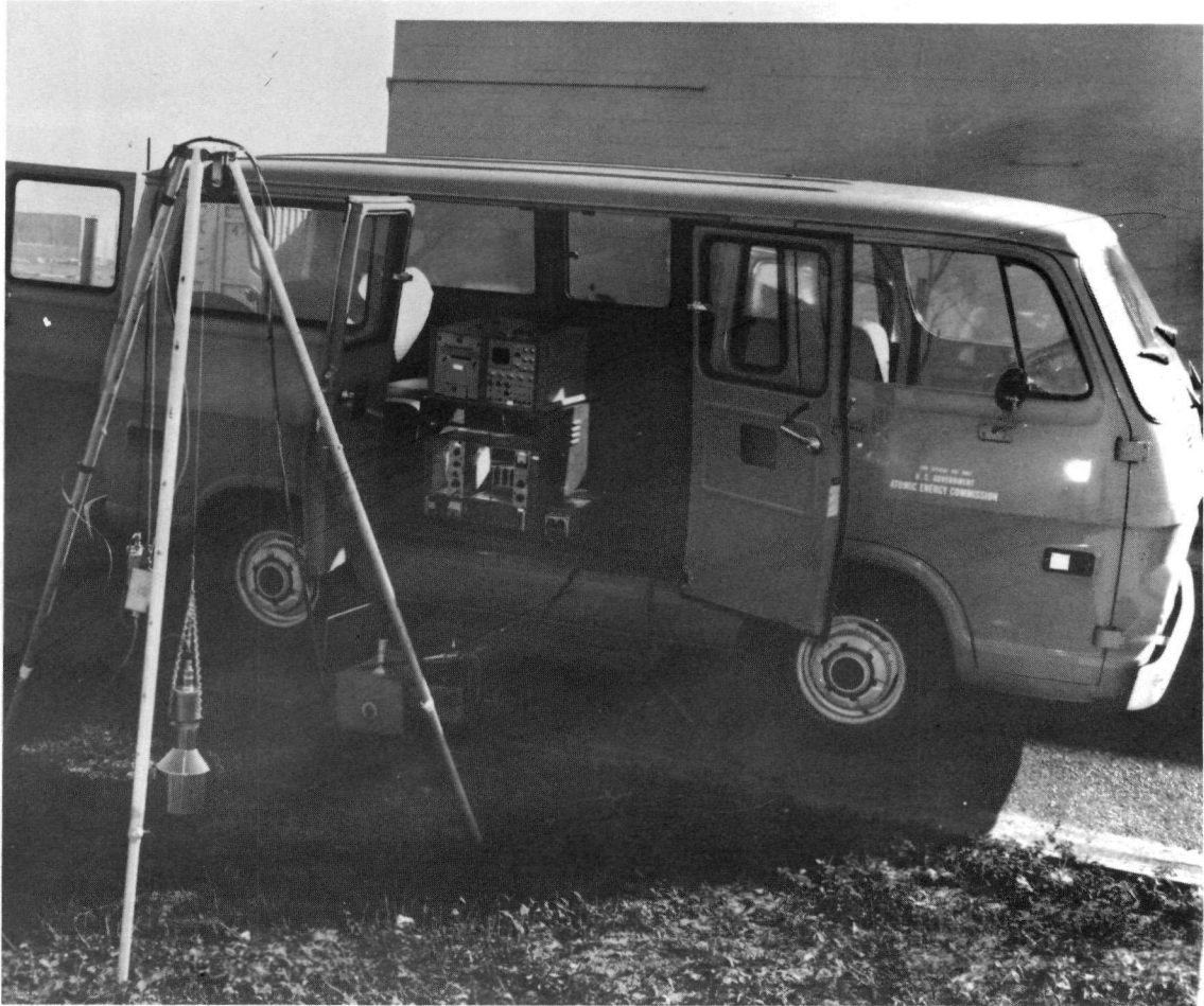
Fig. 2. Field assembly for low-energy terrestrial background spectral measurements using the FIDLER detector.
