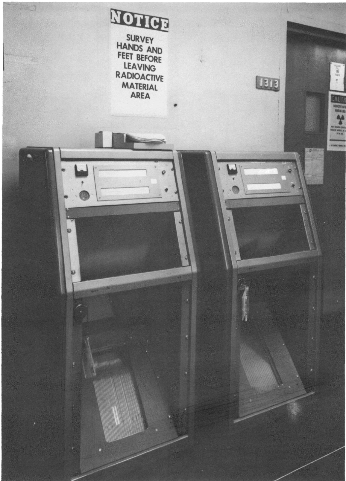
Fig. 3. Hand and foot counter console with audible alarm and visual readout. Note check sources attached by key chains for convenient use.
