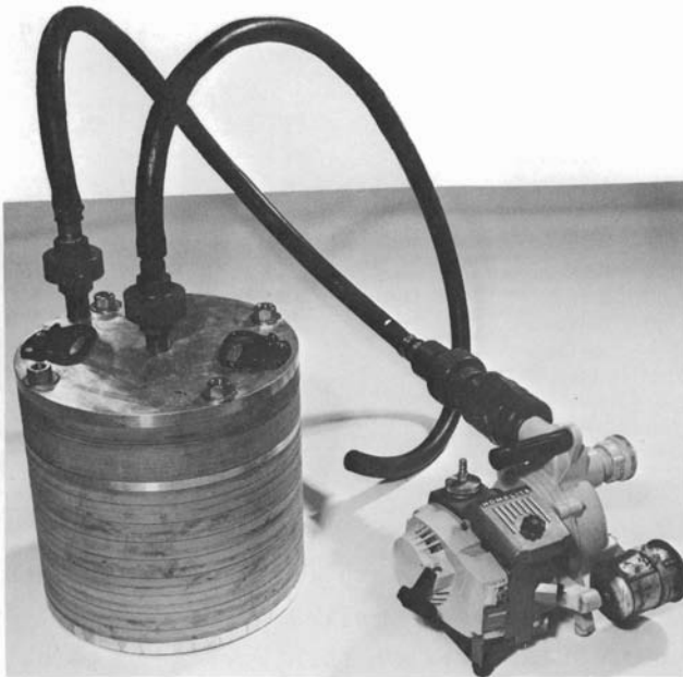
FIGURE 87. Ocean Water Sampling System Showing Assembled PVC Filtration-Sorption Assembly and the High Volume Pump
