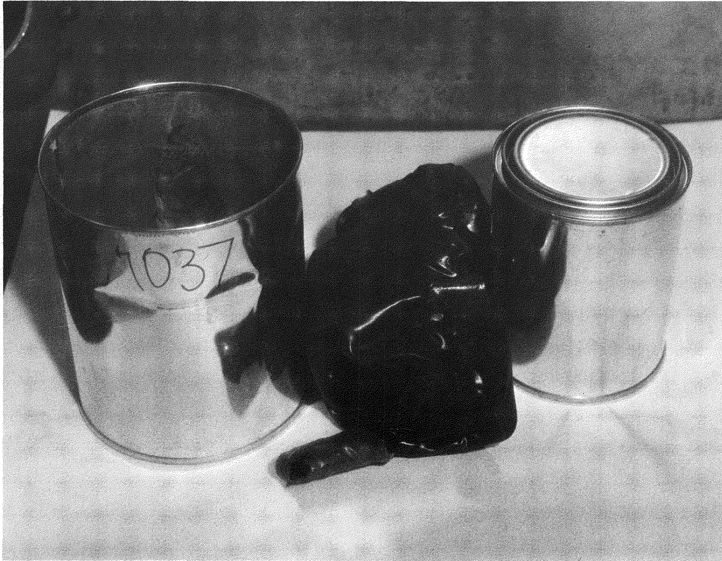
Figure 1. Charred Polyvinyl Chloride Cutout Bag with Containers
