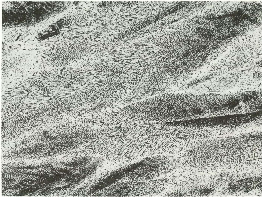
Figure 29. Representative microstructure of the aluminum drop showing the eutectic structure at 760°C in a vacuum atmosphere. Etchant: H 2 O, HF, HNO 3 , HCl. 150X.
