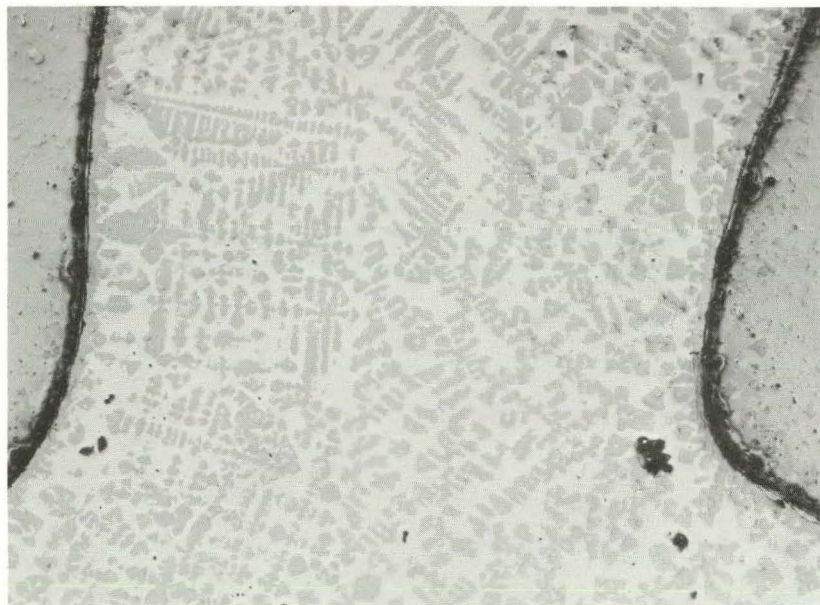
Figure 19. (a) Microstructure of copper drop on beryllium showing interfacial reaction area at 1108^{\circ}\text{C} in a vacuum atmosphere. Unetched. 50X. (b) Microstructure of copper alloying with beryllium at 1108^{\circ}\text{C} in an argon atmosphere. Unetched. 50X.
