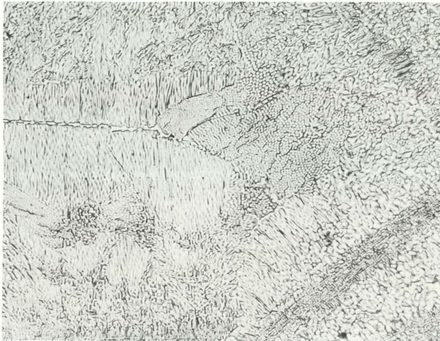
Figure 26. The microstructure of the palladium-beryllium interface area representative of tests in both argon and vacuum at 1030°C. Etchant: aqua regia. 500X.
