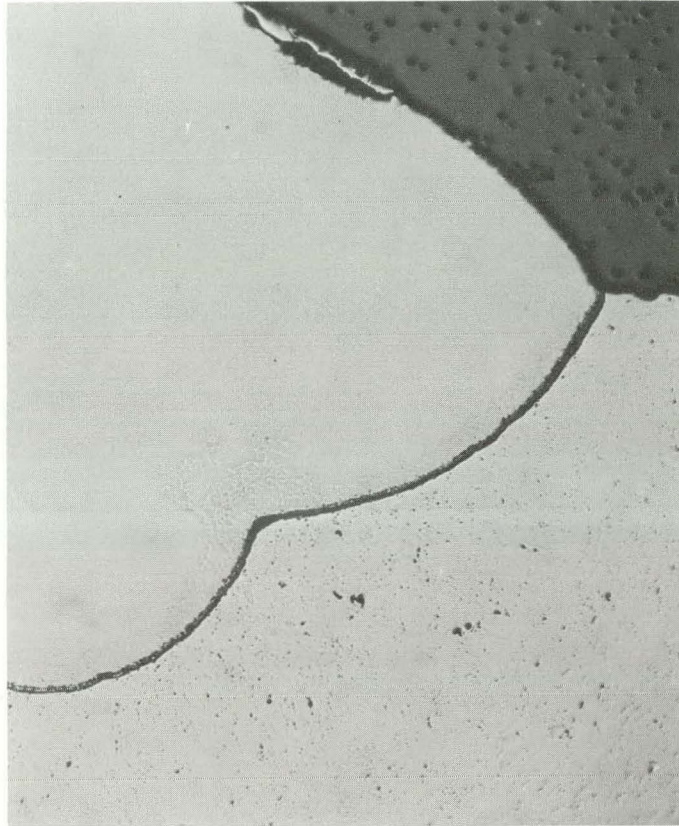
Figure 16. Gold penetration of beryllium metal at 1070°C in a vacuum atmosphere. Unetched. 50X.
