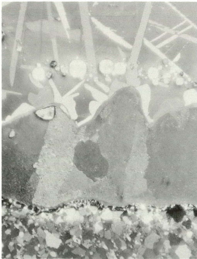
Figure 25. The microstructure of the palladium-2.1 weight per cent beryllium sample interface area representative of tests in both argon and vacuum at 1030°C. Polarized light. 150X.
