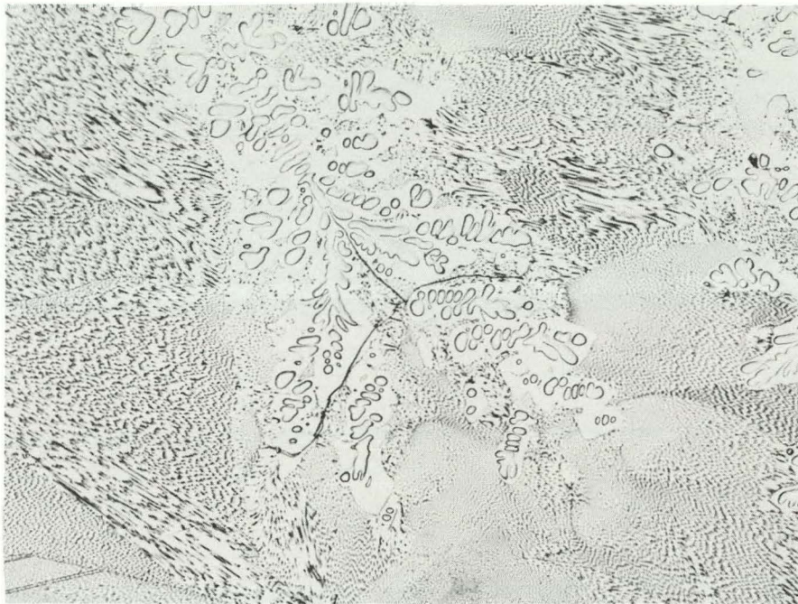
Figure 27. Representative microstructure of the germanium drop at 1000°C in a vacuum atmosphere. Etchant: \text{HC}_2\text{H}_3\text{O}_2 , HF, \text{HNO}_3 . 150X.
