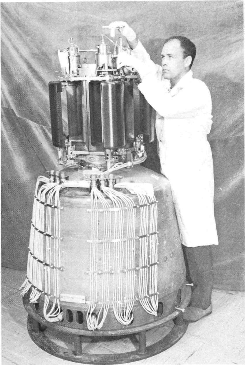
Figure II-79. SNAP 8 Reactor and Shield
