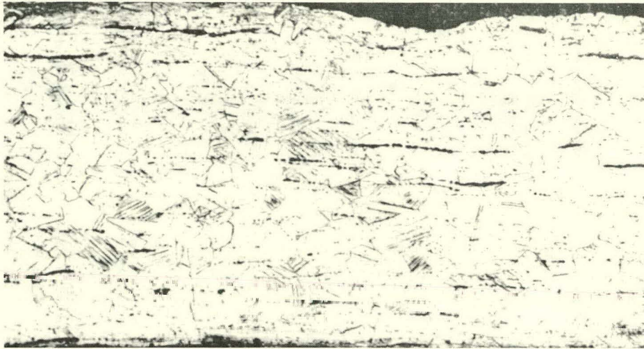
FIGURE 4 COLD SWAGED, PROTOTYPE, LONGITUDINAL SECTION
