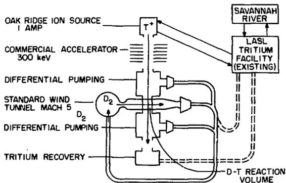
Fig. 11. Schematic of Pump System.
