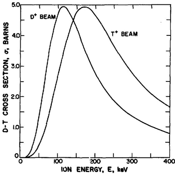
Fig. 2. Neutron production cross section.
