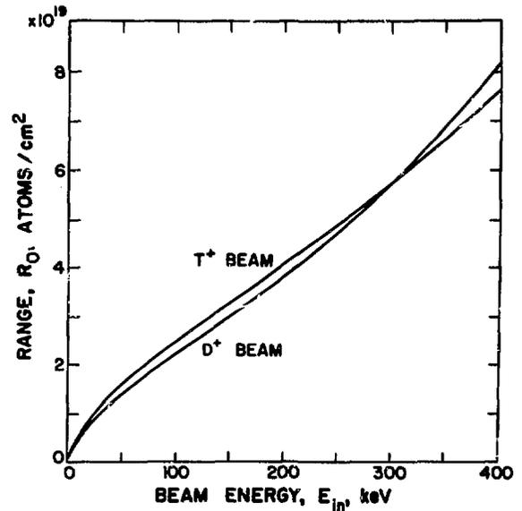
Fig. 5. Ion range for  $D^+$  in  $T_2$  and for  $T^+$  in  $D_2$ .
