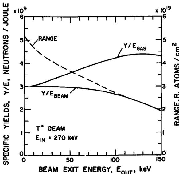
Fig. 7. Specific yield for almost thick target.
