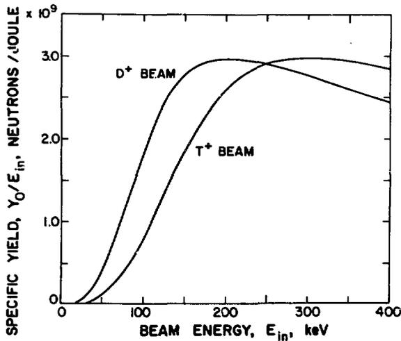
Fig. 6. Specific yield for thick target.
