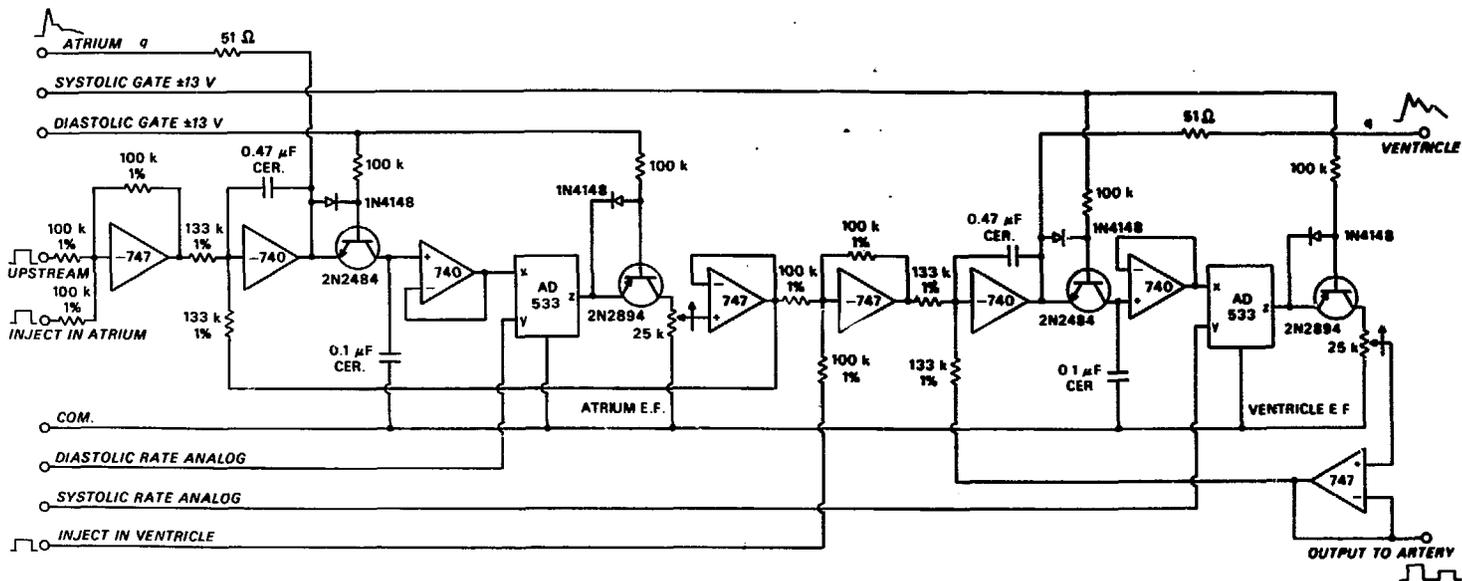
FIG. 13. Diagram of one of the two atrioventricular pairs employed in the analog, showing detail of circuitry and components.
