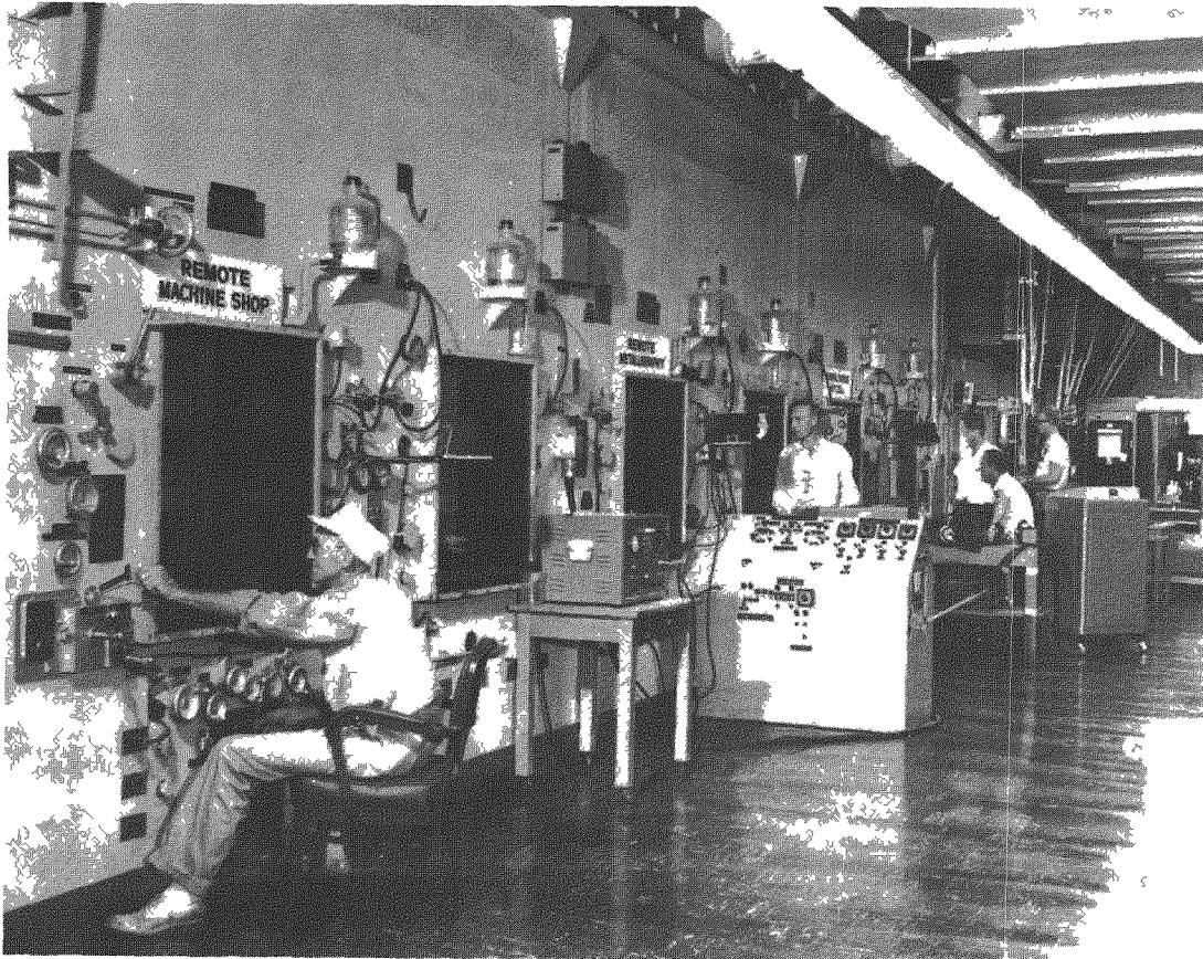
Fig. 37—Operating face of general-purpose hot cells, Solid State Laboratory, building 3025, Oak Ridge
