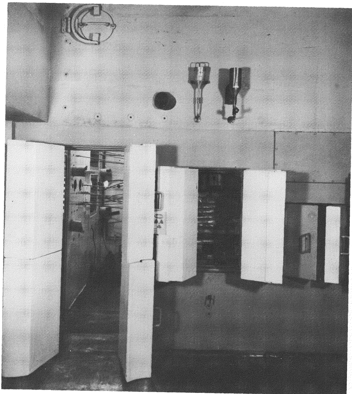
Fig. 32—Access doors to isotope research cell block, High-level Radiochemical Laboratory, building 4501, Oak Ridge.
