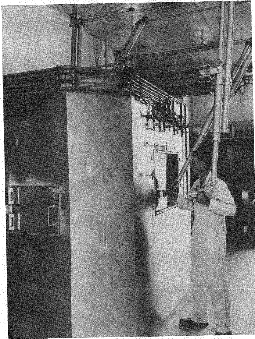
Fig. 46—Operating face of Argonne general-purpose cell, Remote-control Cell Building, 3029, Oak Ridge.
