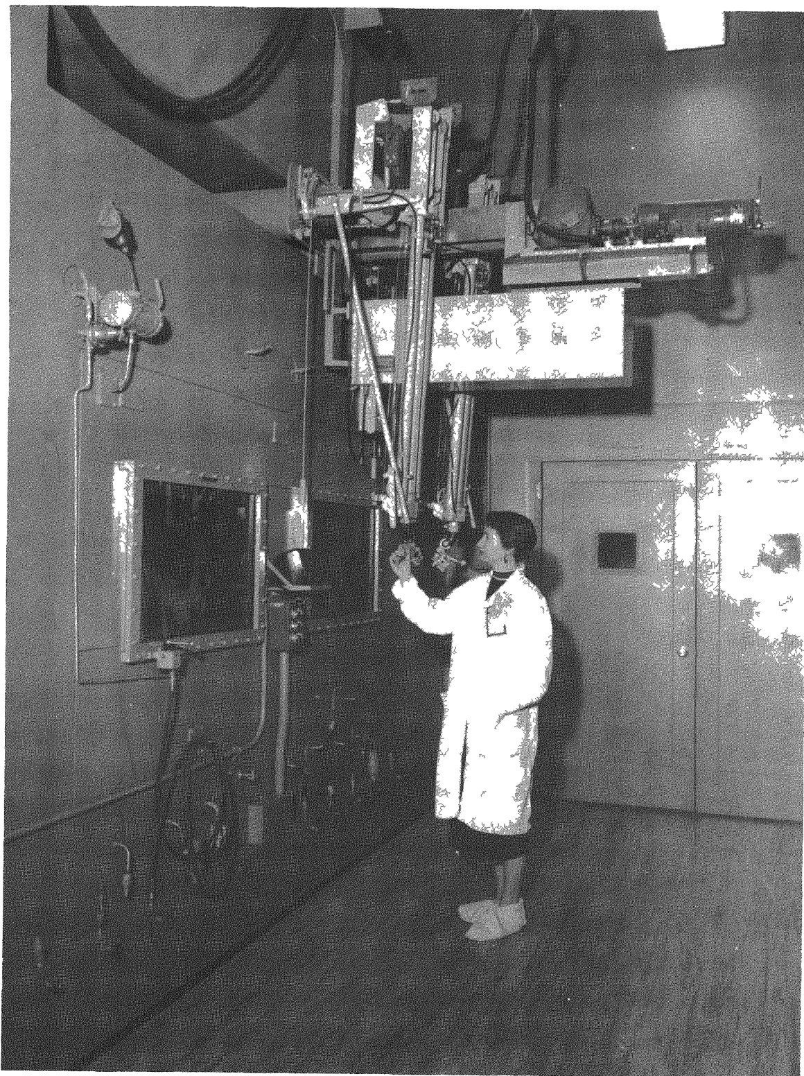
Fig. 20—Operating side of multicurie cell, CPP, Bldg. 627, Idaho.
