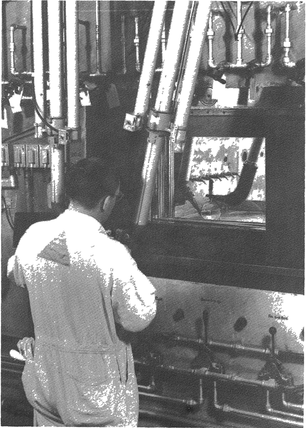
Fig. 43—Operating face of multi-kilocurie loading cell. Remote-control Cell Building, 3029, Oak Ridge.
