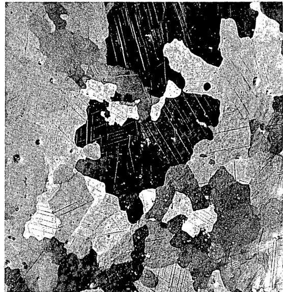
b. After reheating for 120 min at 650°C
