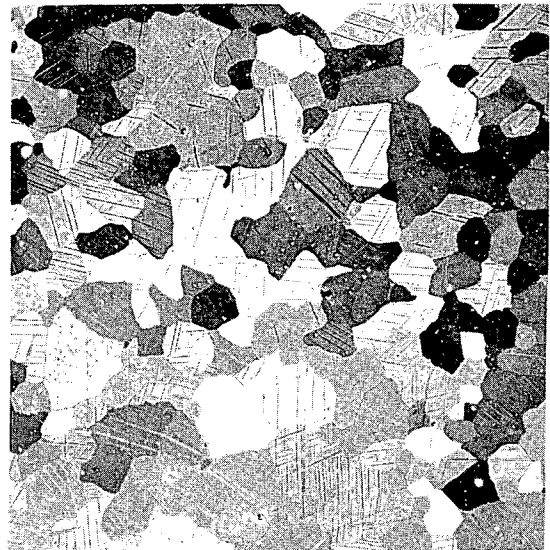
b. Center structure grain size - 0.13 mm
