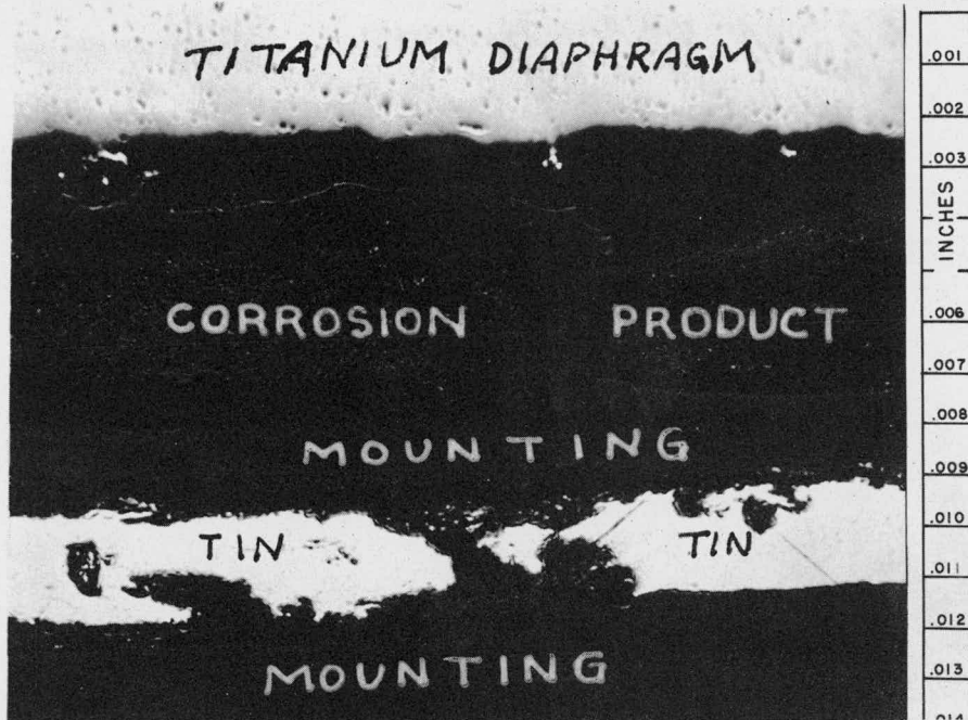
Figure 11 T10367 250X Section Taken at D Shown in Figures 2 and 10
